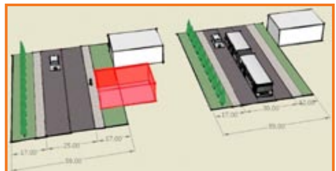
This image illustrates the use of yard setbacks to keep buildings out of a future corridor.
