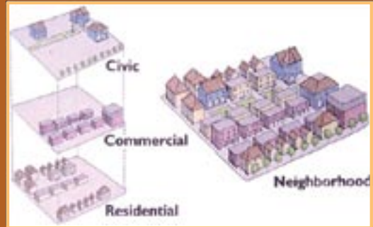
Mixed-use can be either vertical, as in offices above retail, or can be horizontal, such as homes, small-scale retail and offices within a short walk of each other.
